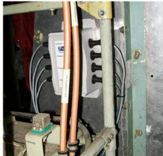
Figure 2: AN110 installed on an aircraft equipment rack
