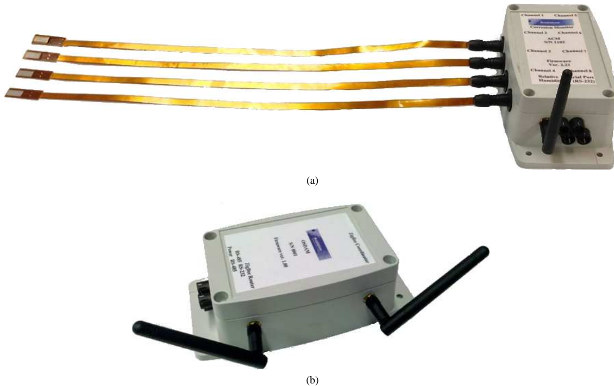
Figure 1.1: Photo of (a) AN110 DAQ node (SHM System) connected to \mu LPR sensors and (b) the Onboard SHM Datastream Aggregator Module (OSDAM)
